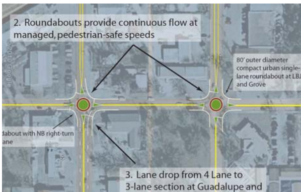
The One-way Couple can be Converted to Two Through Use of Two Roundabouts
